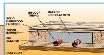
Wood Floor Sleeper System over Infloor Heating
